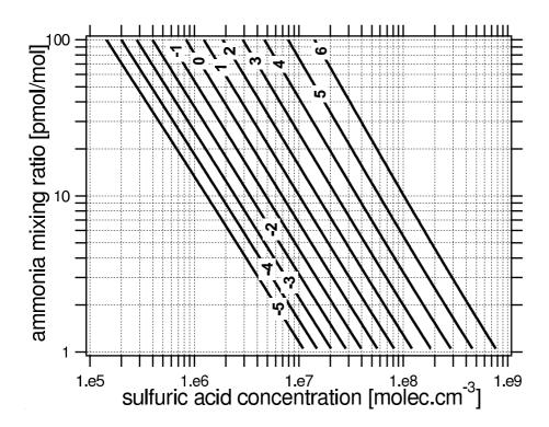
**Fig. 3.** Ternary  $H_2SO_4$ - $NH_3$ - $H_2O$  nucleation rates (isolines labeled with the logarithm of the nucleation rate in nuclei cm<sup>-3</sup> s<sup>-1</sup>) dependent on sulfuric acid concentration and ammonia mixing ratio for fixed temperature (290 K) and fixed relative humidity (63%) as being representative for our sensitivity studies.
