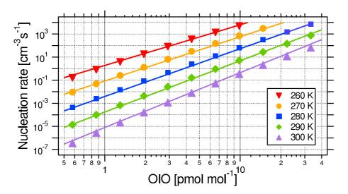
**Fig. 2.** Nucleation rate of 2 nm OIO clusters dependent on OIO mixing ratios for different atmospherically relevant temperatures (symbols). Also displayed are empirical fit functions (solid lines, Eq. 1).
