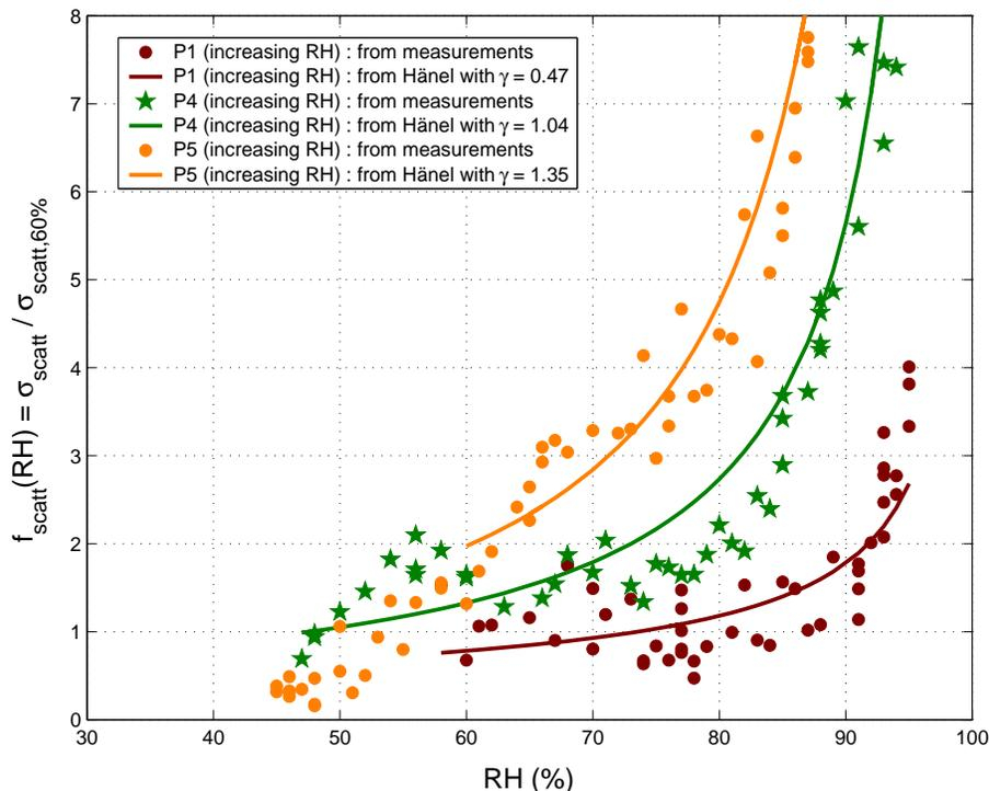
**Fig. 12.** Growth in aerosol scattering cross section as a function of increasing RH for the four time periods P1, P3, P4, and P5. Solid lines represent the Hänel (1976) parameterisation fit of the measurements. Colours identify the sampling filters (see Sect. 4.1). The circle and star symbols indicate a salt mixture of Type 1 and Type 3 (see Sect. 4.2.2).
