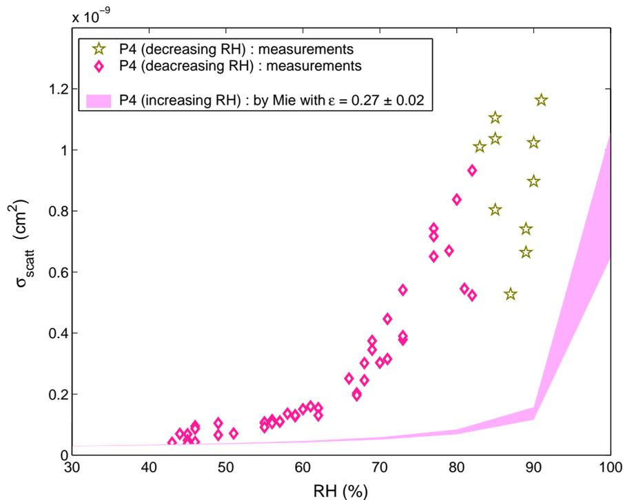
**Fig. 16.** Evidence of the hysteresis phenomenon for the P4 time period. The shaded area corresponds to  $\sigma_{scatt}(\text{RH})$  retrieved from the chemical composition of the aerosols sampled during the decreasing RH  $\sigma_{scatt}(\text{RH})$  measurements (open symbols).
