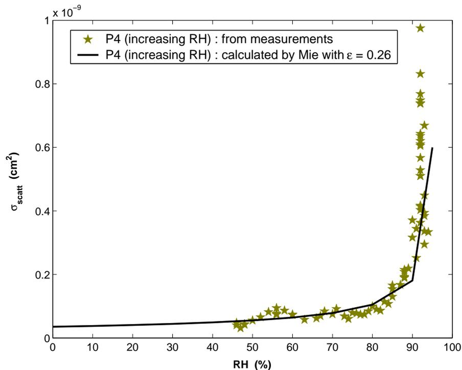
**Fig. 14.**  $\sigma_{scatt}(RH)$  values retrieved from nephelometer measurements and those calculated from Mie theory by using the Hänel growth factor  $\epsilon$ .
