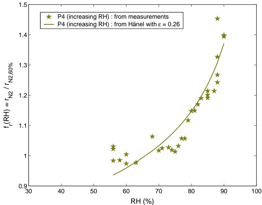
**Fig. 13.** Growth in aerosol size as a function of increasing RH for the P4. Colours identify the sampling filters (see Sect. 4.1). The star symbol indicates a salt mixture of Type 3 (see Sect. 4.2.2). The solid lines represent the Hänel (1976) parameterisation fit of the measurements.
