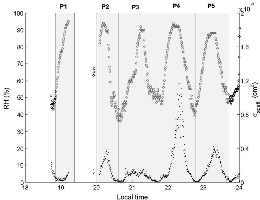
**Fig. 1.** Time evolution of RH (%) (open circles) and of the scattering cross section  $\sigma_{scatt}$  ( $\text{cm}^2$ ) measured at Saclay between 18 and 24 July 2000. The grey areas highlight the 5 time periods (P1, P2, P3, P4, and P5) considered in the text.
