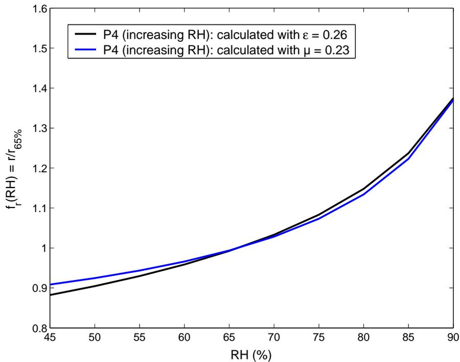
**Fig. 15.** Comparison between  $f_r(\text{RH})$  from number size distributions with  $\epsilon=0.26$  and  $f_r(\text{RH})$  from aerosol water content with  $\mu=0.23$ .
