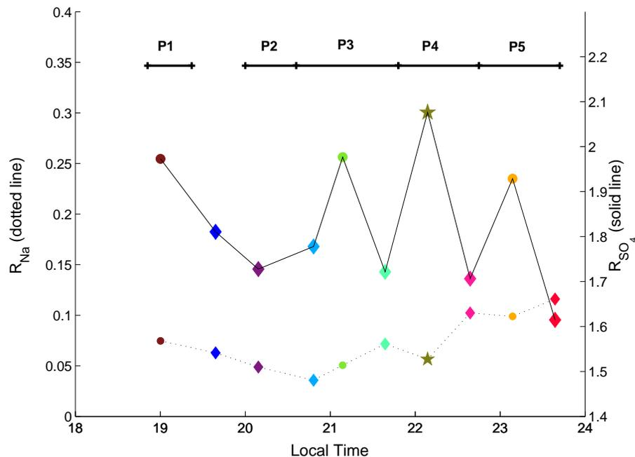
**Fig. 9.** Time evolution of  $R_{\text{SO}_4}$  and  $R_{\text{Na}}$ . The colours identify the sampling filters (see Sect. 4.1). Circle, diamond and star symbols respectively indicate the Type 1, Type 2, and Type 3 pattern of the salt mixture (see Sect. 4.2.2).
