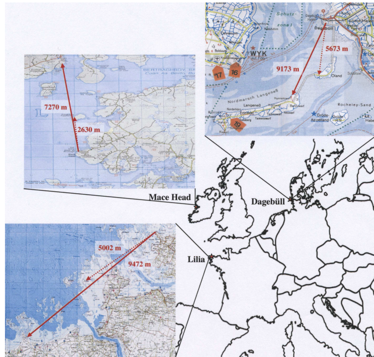
Fig. 2. The three campaign sites Mace Head, Lilia and Dagebüll. The lightpaths are indicated by red arrows. The shorter lightpath (dotted line) was used if the atmospheric conditions didn't allow measurements on the longer one. The shaded areas always indicate the intertidal zones, where the water was removed during low tide. In Dagebüll, as well as, in Lilia the lightpath crossed primarily through the intertidal zone, whereas in Mace Head the lightbeam mainly passed over sea. In the latter location the tidally influenced area with fields of algae is located in easterly direction, e.g. Ard Bay and Bertraghboy Bay.
