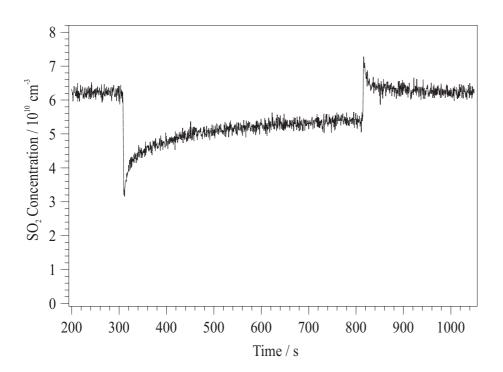
**Fig. 2.** Uptake of  $SO_2$  on an unhumidified Saharan Dust surface at 295 K. The injector was withdrawn 7.4 cm at 310 s to expose  $\sim$ 6.7 mg of dust and returned to its original position at 820 s. Total pressure 1.5 Torr.
