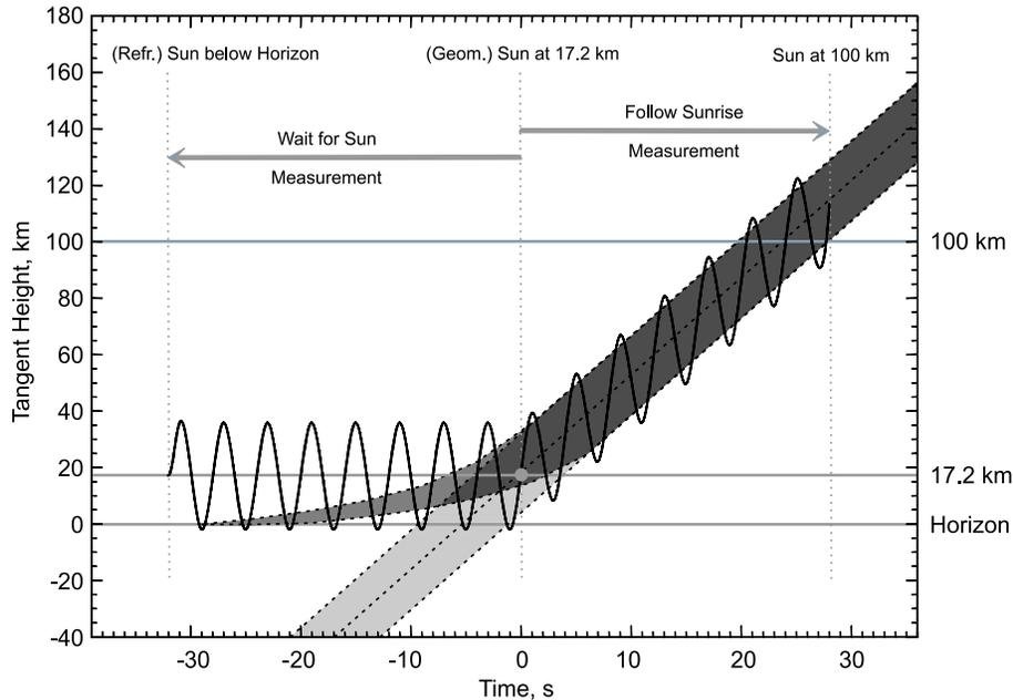
**Fig. 2.** Schematic view of a solar occultation measurement sequence. Tangent height in km is plotted vs. time in seconds. The solid line represents the movement of SCIAMACHY's FOV, the shaded areas illustrate the refracted and the imaginary true sun, respectively.
