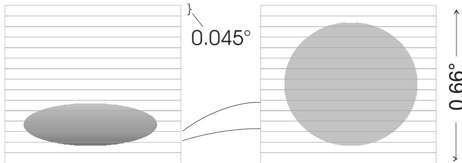
**Fig. 1.** Occultation scan image. SCIAMACHY's fields of view are plotted onto the solar disk for a complete scan. One up or down scan over  $0.66^\circ$  takes two seconds. A typical scan through the atmosphere with refractive effects is shown on the left and a reference scan above the atmosphere is depicted on the right.
