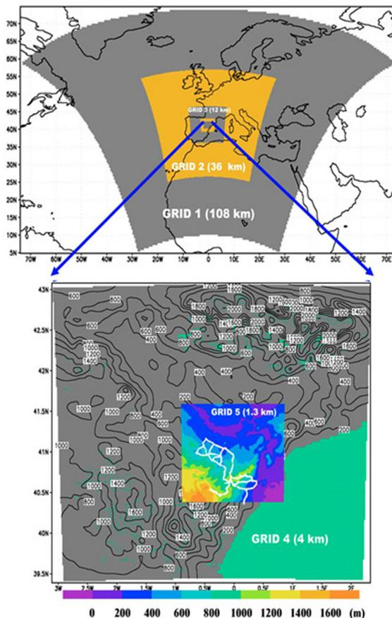
**Fig. 1.** Modelling configuration with the five grids of different resolution employed in the simulations centred over the Andorra power plant ( $G_1$  108 km,  $G_2$  36 km,  $G_3$  12 km,  $G_4$  4 km;  $G_5$  1.3 km). Road network used by the mobile units (instrumented with a COSPEC) to take measurements around the power plant is also indicated in white in the fifth grid.
