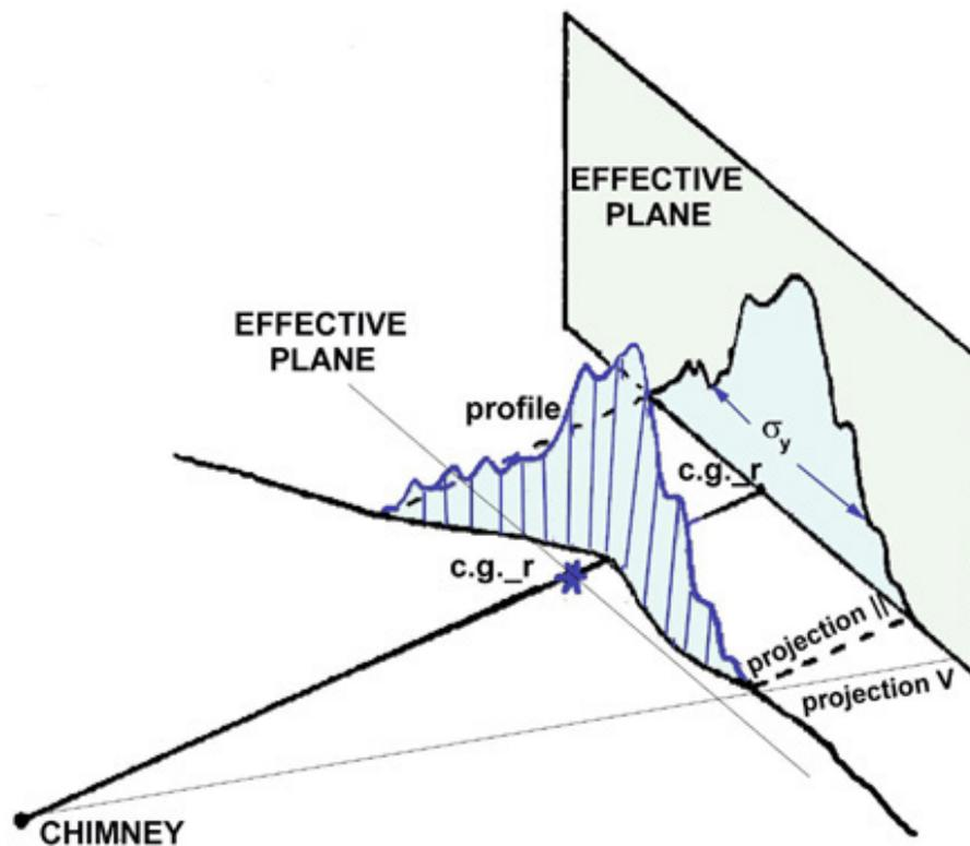
**Fig. A2.** Schematic representation of the definition of “effective plane”, starting from a vertically integrated distribution recorded with the COSPEC along a road span. C.g.\_r is the center of gravity of the distribution measured along the road.
