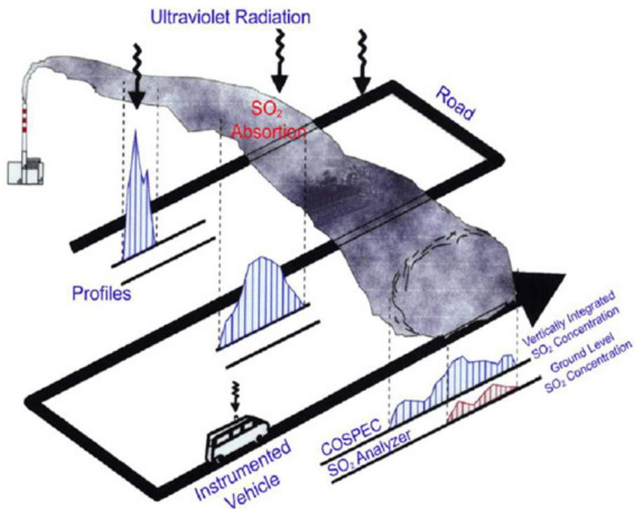
**Fig. A1.** Plume tracking strategy. A vehicle instrumented with a COSPEC and a ground-level analyser makes transects at different distances from the emission source for the whole day.
