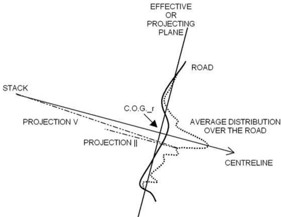
**Fig. A3.** Schematic representation of the definition of the “effective plane” and the “centreline”, starting from a vertically integrated distribution recorded with the COSPEC along a road span. C.g.\_r is the center of gravity of the distribution measured along the road.
