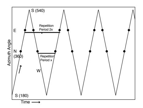
**Fig. 2.** This drawing shows that the repetiton period of a target located in the north (or south) is twice as high as a target located in the east (or west).
