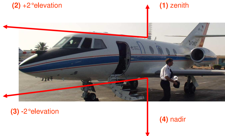
Fig. 2a. Pictures of the DLR-Falcon, including a sketch of the used lines of sights.
