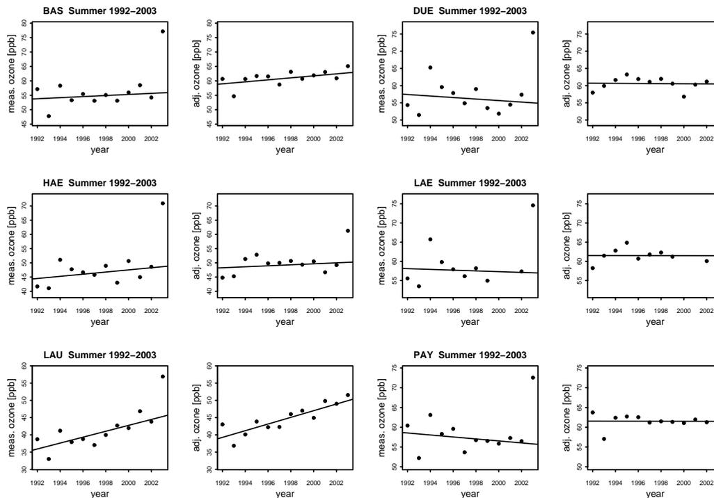
**Fig. 4.** Yearly medians of the daily ozone maxima at the analysed stations in summer for the 1992–2003 period. For every station the first plot shows the yearly median of the measured daily ozone maxima and the second plot depicts the yearly median of the adjusted daily ozone maxima. The trend lines in the plots have been calculated using only summer data from 1992 to 2002.
