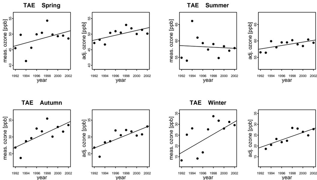
**Fig. 2.** Yearly medians of the measured daily ozone maxima (left) and meteorologically adjusted daily ozone maxima at Tänikon for all seasons during 1992–2002. The calculated MSE ratio ( $MSE_{adj}/MSE_{meas}$ ) for this station is 0.24 in spring, 0.10 in summer, 0.52 in autumn and 0.12 in winter.
