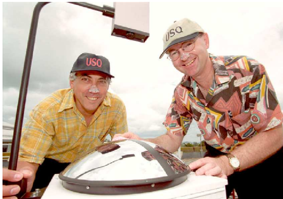
Fig. 1. The TSI-440 at USQ with the first author pictured on the right. The hemispherical dome, shadow band and digital camera can be seen.
