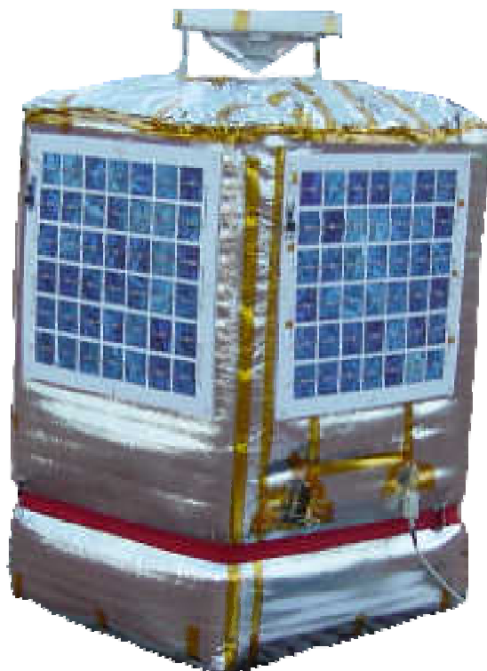
Fig. 1. SAOZ long duration balloon version. The cone at the top of the instruments defines a 360^\circ azimuth, +10^\circ , -10^\circ elevation FOV within which the full sun could be observed at sunrise and sunset without additional tracking system.
