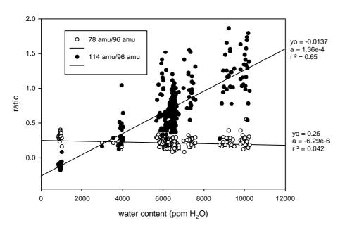
Fig. 4. Ratios of 96/114 and 96/78 amu versus water content of the analyzed air mass during calibration of Acetonitrile.
