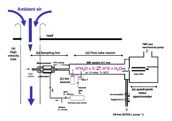
**Fig. 1.** Experimental set up: schematic view of the CIMS instrument. **(a)** high velocity inlet **(b)** critical orifice and sampling line **(c)** ion source, generating  $H_3O^+(H_2O)_n$  educts ions **(d)** flow tube reactor **(e)** quadrupole mass spectrometer.
