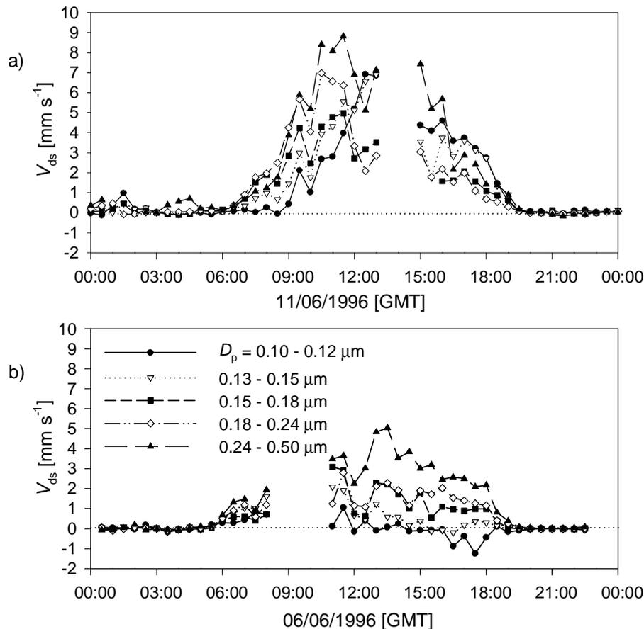
**Fig. 2.** Example daily courses of the deposition velocity of five size classes of particles as measured by eddy-covariance with the ASASP-x. In case (a) particles of all sizes are continuously deposited, at a rate that increases with particle size, whereas (b) on June 6 apparent emission of small particles was observed in the afternoon.
