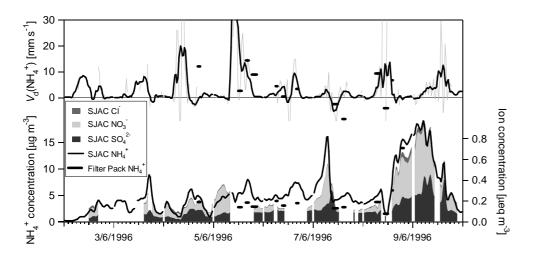
**Fig. 4.** Example time series of  $NH_4^+$  concentrations and deposition velocities ( $V_d$ ) derived by gradient method from the SJAC and filter-pack data. For the SJAC both 30-min measurement data (thin grey) and a 3-h running mean (bold black) are shown. Also shown are the equivalent concentrations of the main anions associated with  $NH_4^+$  ( $SO_4^{2-}$ ,  $NO_3^-$  and  $CI^-$ ).
