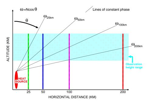
**Fig. 12.** schematic of the wave field observed at the four observation sites denoted by the four colored vertical lines. The range of frequencies observed at each site will correspond roughly to frequencies associated with the steepest and shallowest lines of constant phase that intersect the top and bottom of the observation height range (blue shading).
