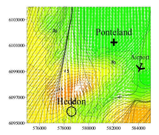
**Fig. 5.** Lincom-T model output (an unstable stratified case). This figure shows the model response to the same wind speed and direction inputs as performed in Fig. 4, but for a case where the temperature stratification (vertical temperature gradient) were deliberately changed from stable (L=+10, c.f. Fig. 4) to unstable (L=-10 m in this figure).
