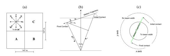
**Fig. 2.** (a) Antenna configuration for interferometric observations of meteors, note that the x-axis is rotated with respect to the East-West baseline  $\sim 51.06^{\circ}$ . Simplified geometry of a meteor trajectory respect to the illuminated beam: (b) altitudinal and (c) horizontal views.
