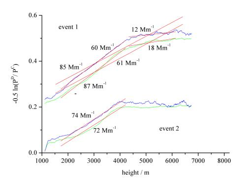
**Fig. 2.** Retrieval of the extinction of the Saharan dust clouds by determining the slope of the ratio of two Raman profiles. Extinction in the lower layer of event 1 (upper curves) are higher than the overall mean.
