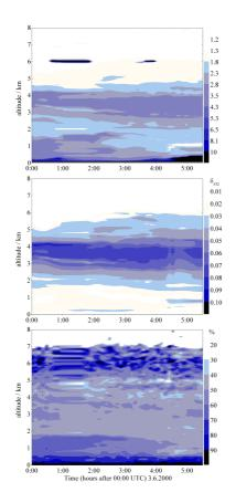
**Fig. 3.** Backscatter ratio (upper) and volume depolarization (middle panel) at 532 nm as well as relative humidity measured by the Raman lidar (lower panel) on 3 June 2000 around 10° N 22° W. The Saharan dust layer extends from 2 km up to 6 km.
