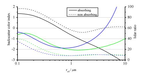
**Fig. 7.** Behavior of the color index (black) and the lidar ratio (blue for 355 nm, green at 355 nm) according to Mie calculation using the refractive indices given by Dubovik et al. (2002). For comparison the dotted lines give the same quantities for refractive indices with an imaginary part k = 0.
