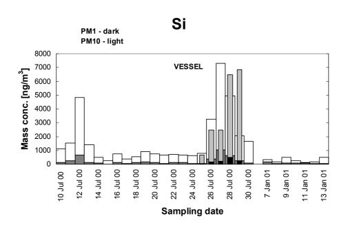
**Fig. 3.** (a) Daily concentrations of (a) Si, (b) K, (c) Cl, (d) S, and (e) V in PM1 and PM10 at Finokalia and aboard of the research vessel "AEGAIEO".
