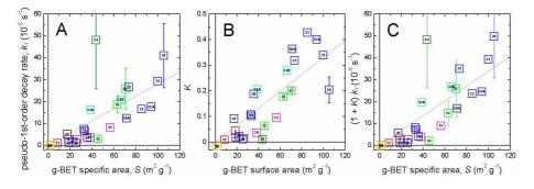
**Fig. 5. (A)** Pseudo-first-order rate constant  $k_1$ , **(B)** removal ratio due to the adsorption K, and **(C)** (1+K)  $k_1$  in reactions on various API standard clay minerals at 313 K versus specific surface area S of each clay mineral deduced by Eq. (2). The label indicates the API number of the clay minerals. Clay minerals of the same type are represented by the same color.
