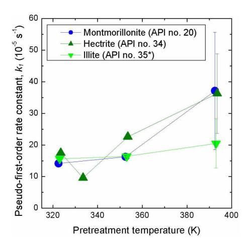
**Fig. 7.** The pseudo-first-order reaction rate in reactions on clay minerals at 313 K versus the pretreatment temperature of clay minerals. The pretreatment temperature means the temperature at which montmorillonite (API no. 20), hectorite (API no. 34), or illite (API no. 35\*) was heated before the reaction.
