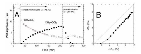
**Fig. 3.** Changes in  $CH_3CCl_3$  and newly formed  $CH_2=CCl_2$  for the reaction shown in Fig. 2. **(A)** Time course of  $CH_3CCl_3$  (open symbol) and newly formed  $CH_2=CCl_2$  (solid symbol) partial pressures. Solid red line is a fit by first-order kinetics. **(B)** The decrease in  $CH_3CCl_3$  partial pressure  $(-\Delta P_{MC})$  versus the increase in  $CH_2=CCl_2$  partial pressure  $(\Delta P_{DE})$  during a 180-min reaction without photoillumination.
