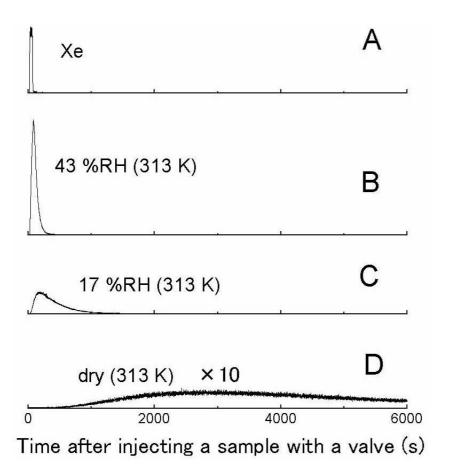
**Fig. 13.** The results of the column experiment for illite (no.  $35^*$ ) in dry or humidified He flow at 313 K. **(A)** The experiment of a Xe-He mixture in dry He flow. **(B)–(D)** The experiments of a  $CH_3CCI_3He$  mixture in (B) 43% RH, (C) 17% RH, and (D) dry He flow.
