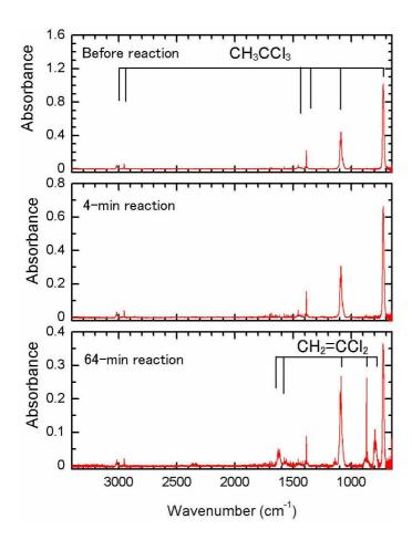
**Fig. 2.** IR spectra of  $CH_3CCI_3$  and its decomposition products in the gas phase for the reaction of  $CH_3CCI_3$  in air on halloysite (API no. 12) particles at 313 K. **(a)** Before contact with the halloysite, **(b)** after a 4-min, and **(c)** after a 64-min reaction.
