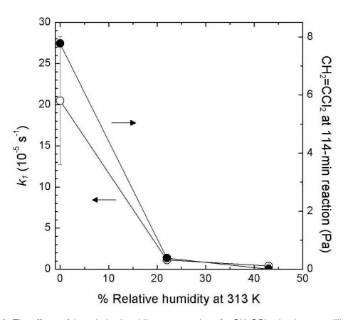
**Fig. 12.** The effects of the relative humidity on a reaction of a  $CH_3CCl_3$ -air mixture on illite (API no. 35\*) materials at 313 K. Open symbols represent the pseudo-first-order rate constant; solid symbols represent the amount of  $CH_2=CCl_2$  produced in a 114-min reaction.
