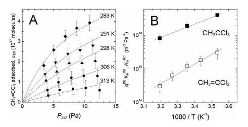
**Fig. 10.** Adsorption on illite (API no. 35\*). **(A)** Isotherms of  $CH_2 = CCI_2$  in air at 283–313 K. **(B)** The temperature dependence of the adsorption parameters for  $CH_2 = CCI_2$  (open symbols) and  $CH_3CCI_3$  (solid symbols).
