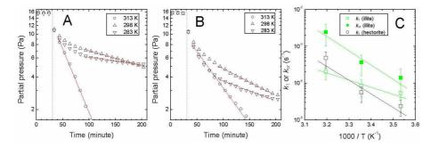
**Fig. 8. (A)** Semi-log plot of the time course of  $CH_3CCl_3$  partial pressures for the reactions on hectorite (API no. 34) and **(B)** on illite (API no. 35\*) at 283–313 K. **(C)** The  $k_1$  values averaged for the reaction on hectorite (API no. 34) and the  $k_1$  and  $k_{sr}$  values averaged for the reaction on illite (API no. 35\*) versus the inverse of reaction temperatures; open square,  $k_1$ ; solid square,  $k_{sr}$ .
