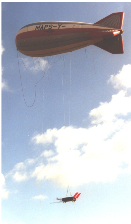
Fig. 3. The tethered-balloon MAPS-Y with the suspended payload ACTOS.
