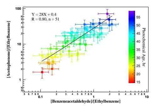
**Fig.7.** Correlation between the ratios [acetophenone]/[ethylbenzene] and [benzeneacetalde-hyde]/[ethylbenzene]. The vertical and horizontal bars represent the estimated errors in the ratios. Photochemical ages, as derived from the [acetophenone]/[ethylbenzene] ratios, are coded in color.
