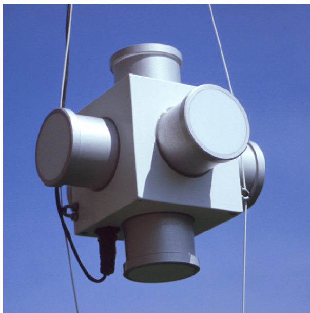
Fig. 1. The NILU-CUBE before being protected by styrofoam. The size is about 18 cm from head to head. The weight, including a separate data logging unit is less than 4 kg.
