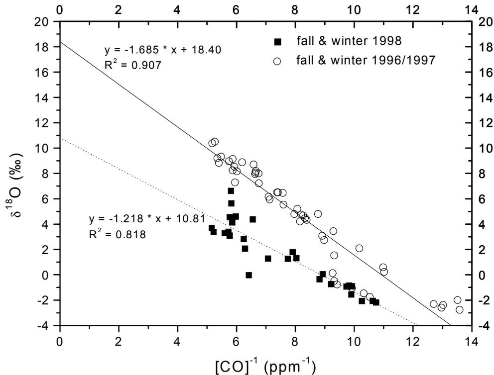
**Fig. 3.** The correlation plot of fall and winter  $\delta^{18}\text{O}$  data versus inverse CO mixing ratio showing a clear difference between the “normal” years 1996 and 1997, and 1998 with the CO anomaly. The low  $y$ -axis intercept has been found to be indicative of CO from biomass burning in boreal forest regions in several recent studies.
