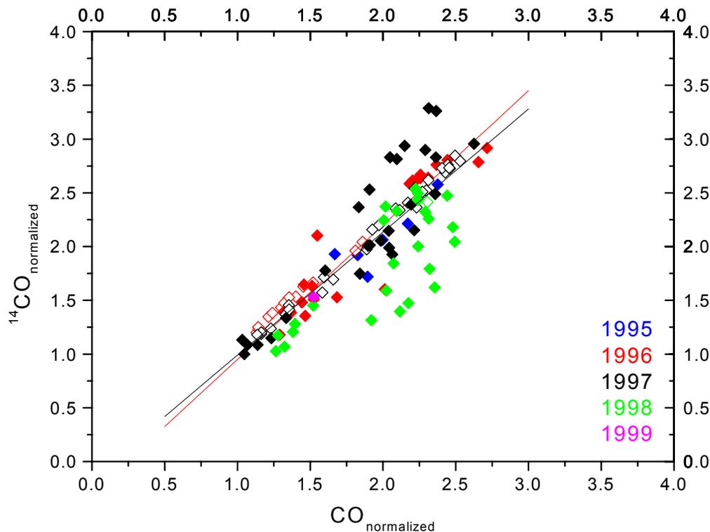
**Fig. 2.** Normalized  $^{14}\text{CO}$  values vs. normalized CO. The original data have been normalized by dividing through the  $^{14}\text{CO}$  and CO minimum values. Linear fits are applied to the 1996 data (red line) and to all data (black line).
