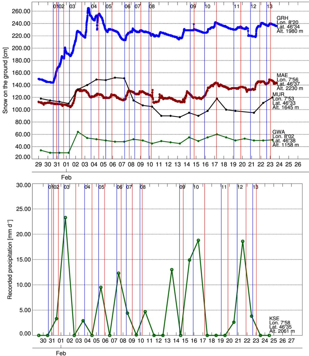
Figure 4: Top panel: snow height measurements during CLACE2014 in 4 different automatic stations. Bottom panel: daily accumulation of liquid water measured at the KS site.
