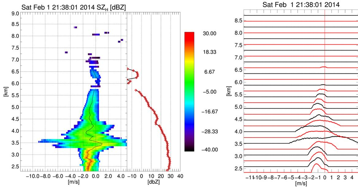
Figure 3: Example of a Doppler spectrum (spectral reflectivity factor) collected at vertical incidence during EV3. Left: color-coded Doppler spectrum, and right: stacked spectra.
