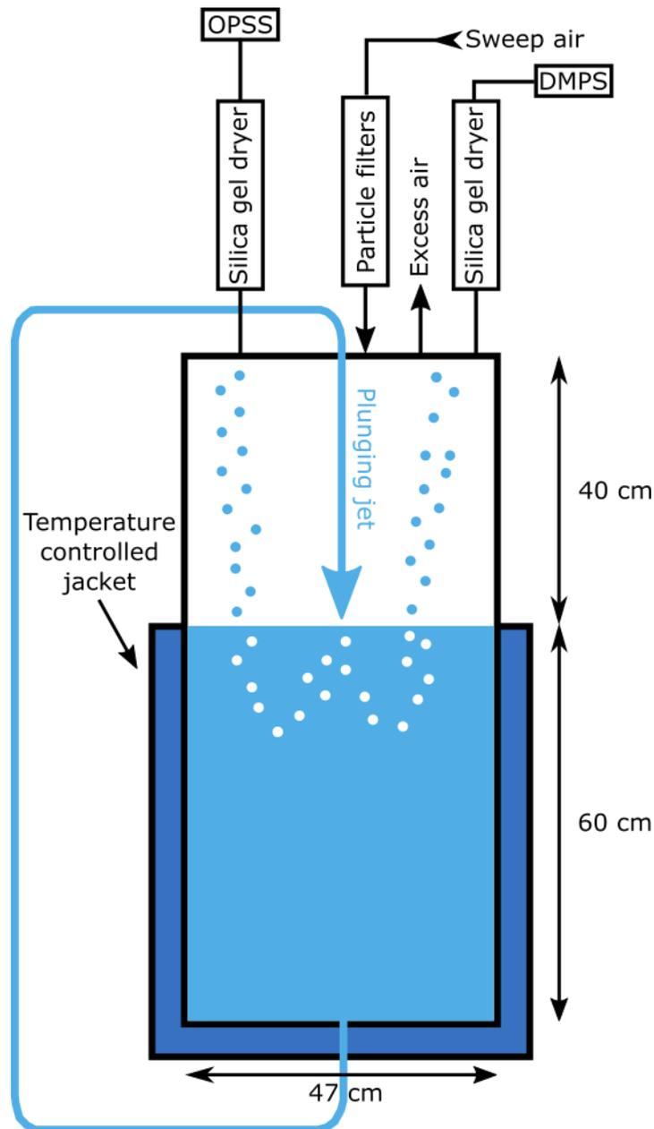
Figure 3: Schematic of the plunging jet tank used for the experiments.
