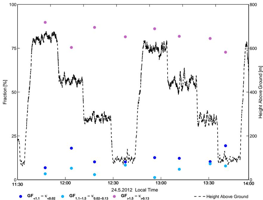
**Figure 12.** Time evolution of the mixing state of the aerosol particles (with  $D_{\text{dry}} = 500 \text{ nm}$ ) for the height profiles near Cabauw on 24 May 2012. Particles are classified into three hygroscopicity categories according to their GF (equally defined as for Fig. 4):  $GF < 1.1$ ,  $1.1 < GF < 1.5$ ,  $GF > 1.5$ , in blue, light blue and pink respectively; these correspond to  $\kappa < 0.02$ ,  $0.02 < \kappa < 0.13$  and  $\kappa > 0.13$ .
