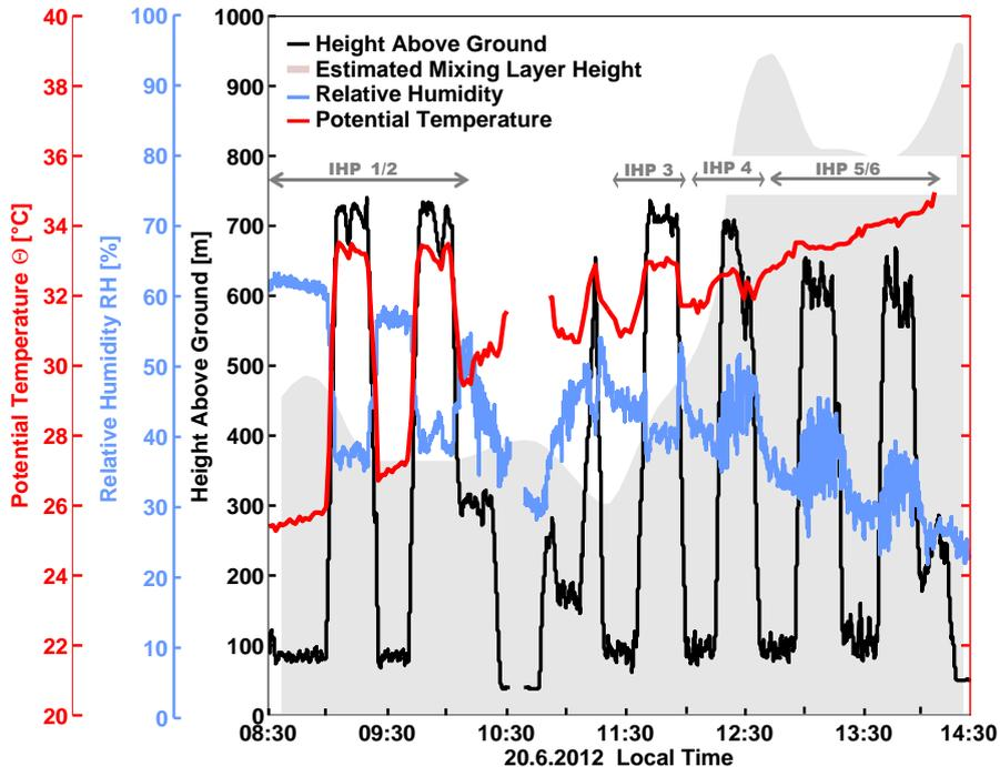
**Figure 2.** Overview of the flight on 20 June 2012 near San Pietro Capofiume ground station (Po Valley, Italy). In black the flight altitude and in grey the estimated mixing layer height, determined from ceilometer – Lidar measurements, are presented. The red and blue lines show the potential temperature  $\Theta$  and RH profiles, respectively. In addition, the different height profiles IHP1/2, IHP3, IHP4 and IHP5/6 are indicated.
