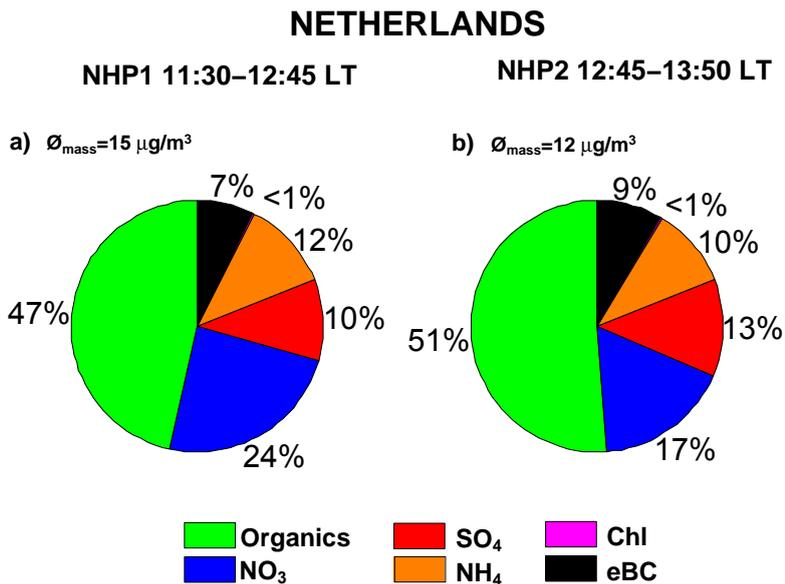
**Figure 10.** Ground measurements of the aerosol particle chemical composition at the Cabauw tower during NHP1 and NHP2 on 24 May 2012. HR-ToF-AMS and MAAP results are combined for the total aerosol mass. Also, the averaged mass concentrations during the profile periods are stated.
