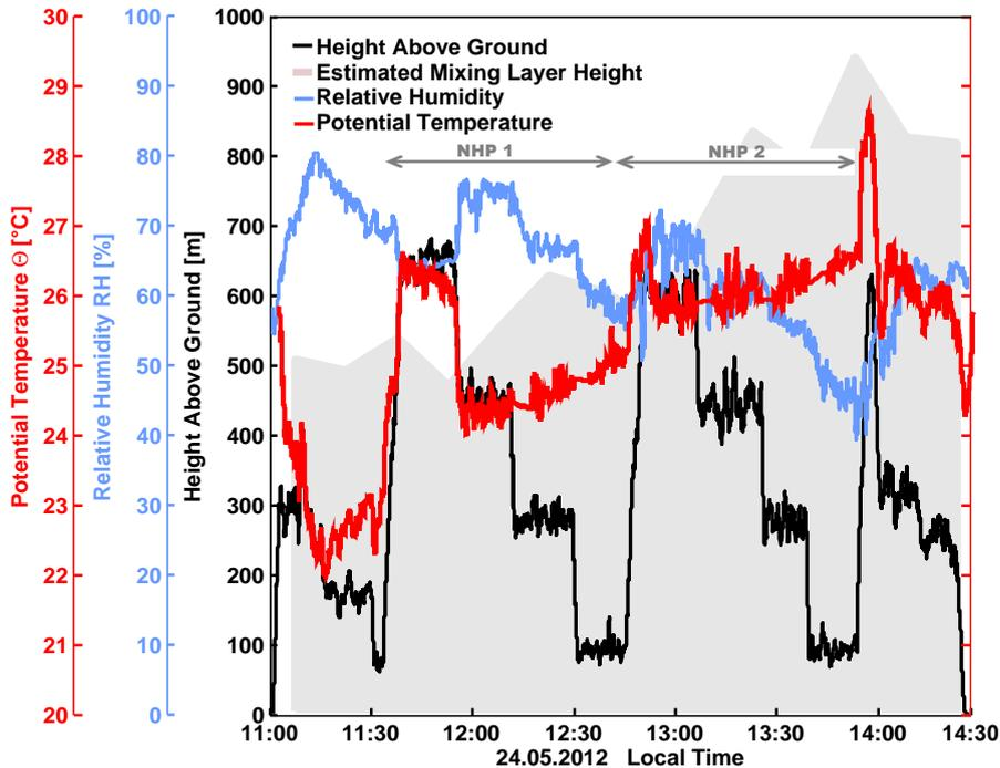
**Figure 9.** Overview of the flight on 24 May 2012 near the Cabauw CESAR station in the Netherlands. In black the flight altitude and in grey the estimated mixing layer height, inferred from ceilometer measurements, are presented. The red and blue lines show the potential temperature  $\Theta$  and RH profiles, respectively. In addition, the different height profiles NHP1 and NHP2 are indicated.
