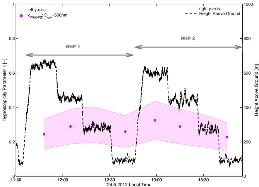
**Figure 13.** Time series of  $\kappa$  values retrieved during the flight on 24 May 2012. WHOPS results for a dry diameter of 500 nm are presented. The measurement accuracy is shown as the shaded area. Additionally, the flight altitude is indicated.
