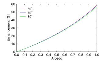
**Figure 2.** Enhancement of the clear-sky UVI as a function of albedo. The plot is based on radiative transfer calculations with the libRadtran model (Mayer and Kylling, 2005) for sea level, a TOC of 400 DU, and SZAs of 60°, 70° and 80° as indicated in the legend.
