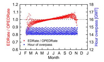
**Figure 9.** Ratio of EDRate/OPEDRate from OMI data file (red, left axis) and the hour of the OMI overpass (blue, right axis) derived from the Summit dataset. Data were filtered for VZA <  $20^{\circ}$ . The ticks on the *x* axis indicate the start of a given month.
