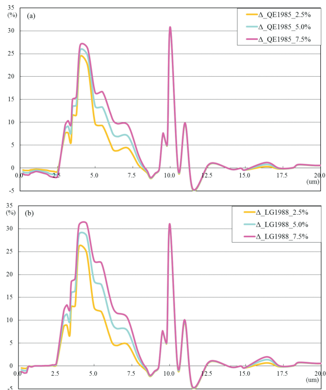
Figure 6. The difference \Delta\omega_0 between the single scattering albedo (SSA) of pure illite and the single scattering albedo of mixtures with different contents and refractive indices of hematite. (a) Complex refractive index of hematite from Qurrey (1985), (b) complex refractive index of hematite from Longtin (1988).
