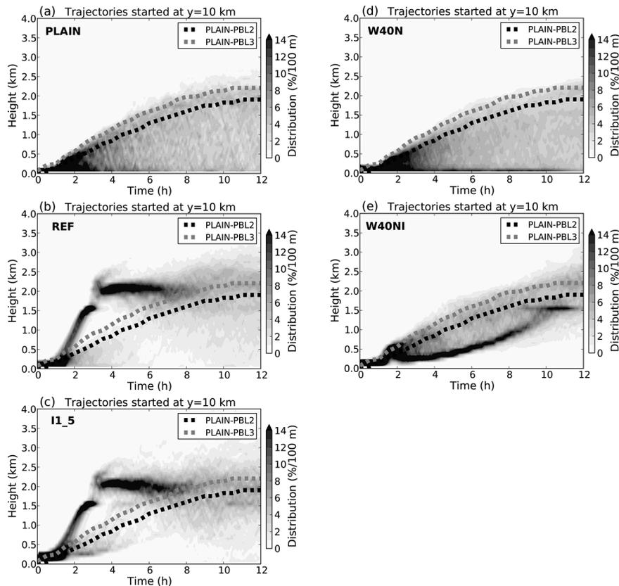
**Figure 11.** Evolution of parcel height distribution for trajectories started at  $y = 10$  km for **(a)** PLAIN, **(b)** REF, **(c)** I1\_5, **(d)** W40N and **(e)** W40NI simulation. The thick black and grey dashed lines mark the PLAIN-PBL2 and PLAIN-PBL3 height, respectively. Distribution values are calculated by splitting the vertical height column into bins of 100 m and determining the percentage of parcels within these height intervals ( $\% 100 \text{ m}^{-1}$ ).
