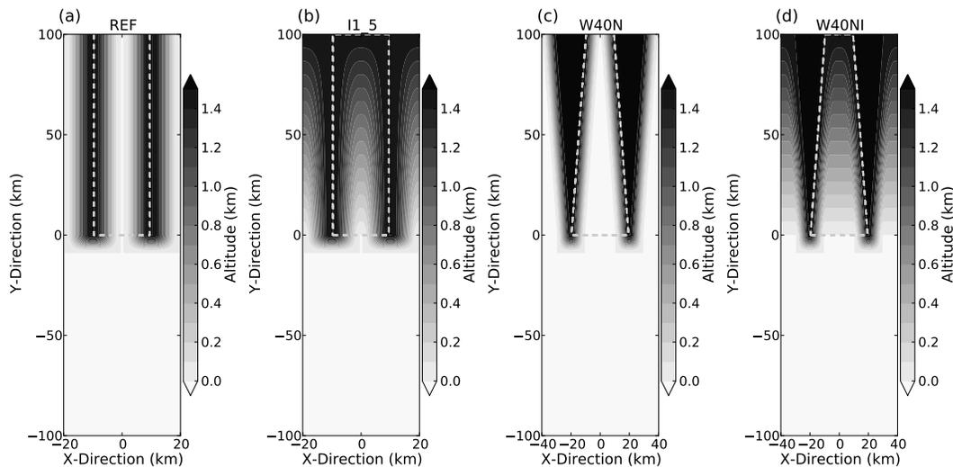
**Figure 1.** Modelling domain and valley topography for **(a)** REF, **(b)** I1\_5, **(c)** W40N and **(d)** W40NI simulations. The dashed grey boxes mark the horizontal areas at crest height, which define the upper surface of a box that is used for computations of valley volume mass flux budgets and valley volume averages of along-valley wind speed.
