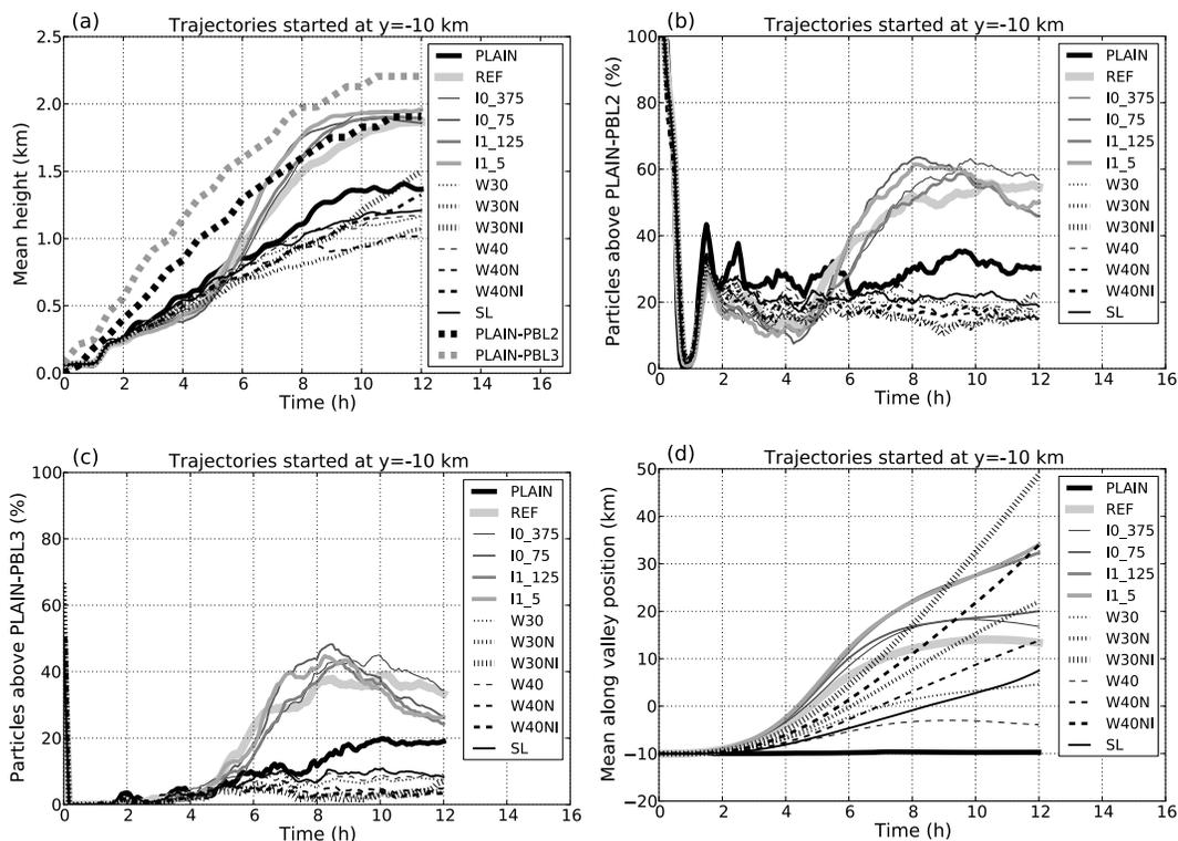
**Figure 14.** Time series of (a) mean trajectory height, (b) fraction of parcels, which are located above PLAIN-PBL2 and (c) above PLAIN-PBL3 and (d) mean along-valley position of parcels started at  $y = -10$  km. The thick black and grey dashed lines in (a) mark the PLAIN-PBL2 and PLAIN-PBL3 height, respectively.
