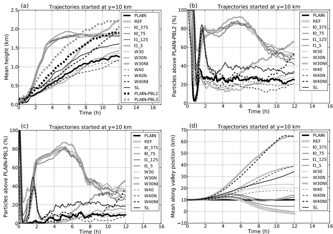
**Figure 13.** Time series of (a) mean trajectory height, (b) fraction of parcels, which are located above PLAIN-PBL2 and (c) above PLAIN-PBL3 and (d) mean along-valley position of parcels started at  $y = 10$  km. The thick black and grey dashed lines in (a) mark the PLAIN-PBL2 and PLAIN-PBL3 height, respectively.
