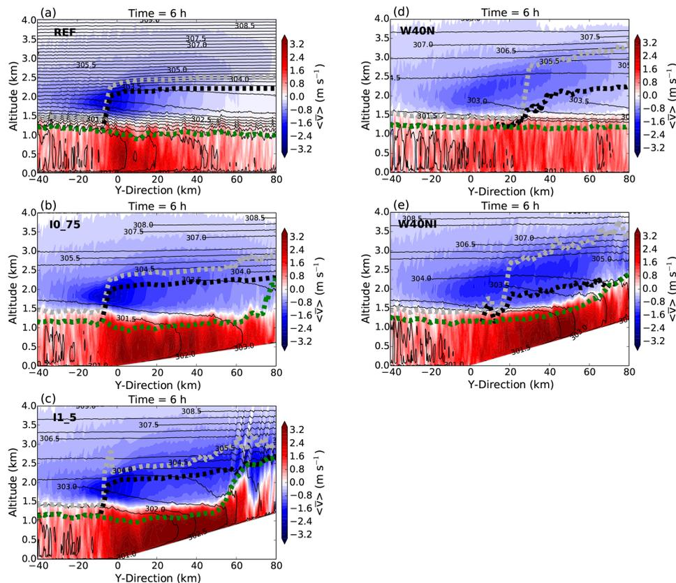
**Figure 5.** Temporally averaged along-valley flow (colour shading) and potential temperature (contour lines) after 6 h of simulation at  $x = 0$  km for different valley depths and widths. Boundary layer heights PBL1, PBL2 and PBL3 are plotted with thick dashed green, black and grey lines, respectively.
