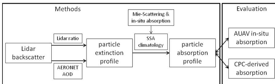
**Figure 1.** Flow chart describing the derivation of particle absorption profiles from lidar measurements, and their evaluation against in-situ observations.
