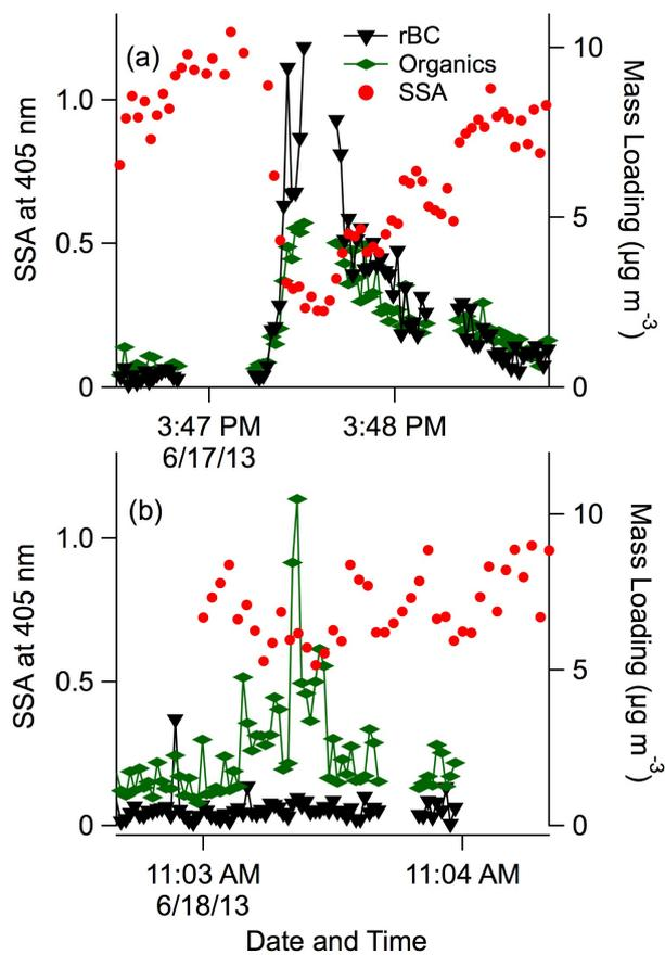
**Figure 6.** Examples of rBC-dominated (a) and organic-dominated (b) plumes observed using the SP-AMS with high-time resolution (1 Hz) sampling, with measurements of single scattering albedo (SSA) at 405 nm from a photoacoustic soot spectrometer (PASS-3). Gaps in SP-AMS data correspond to periods used for the subtraction of gas-phase contributions from particle signals. Mass spectra shown in Figure 1(g) and (h) correspond to plumes in (b) and (a), respectively.
