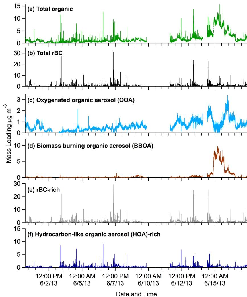
**Figure 5.** Time series of (a) ensemble organic aerosol and (b) refractory black carbon mass loadings during the roadside study. Positive matrix factorization (PMF) results for ensemble data (c) to (f): (c) regionally sourced rBC mixed with oxygenated organic aerosol, (d) biomass-burning organic aerosol mixed with rBC, and traffic-related rBC in an rBC-rich and HOA-rich factor (e) and (f). Mass spectra of all PMF factors are shown in Fig. S1 in the Supplement.
