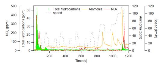
Figure 4. Time-series of the exhaust concentrations of total hydrocarbons, ammonia and NO<sub>x</sub>.
