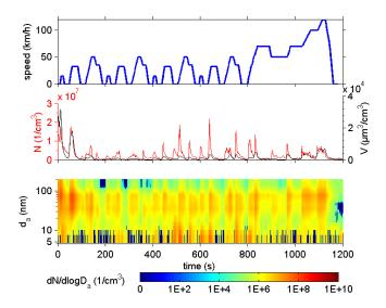
Figure 2. Speed profile, primary particle number (measured by the CPC) and volume concentrations (measured by HRLPI) and primary particle size distributions (HRLPI) for the studied gasoline passenger car during the NEDC test cycle.
