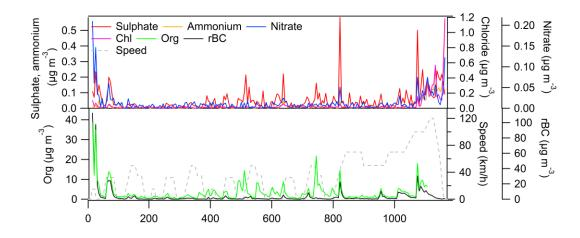
Figure 3. Temporal behavior of rBC, organics, SO<sub>4</sub>, NO<sub>3</sub> and NH<sub>4</sub> concentrations measured by the SP-AMS for the primary emissions (without the PAM chamber) during the NEDC test cycle.
