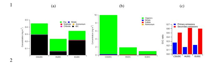
Figure 7. (a) Chemical composition of primary PM, (b) chemical composition secondary PM, and (c) the O:C –ratios of primary and secondary particulate matter for different parts of the NEDC cycle.
