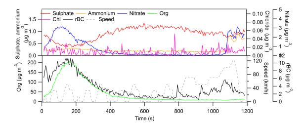
Figure 6. Temporal behavior of rBC, organics, SO<sub>4</sub>, NO<sub>3</sub>, NH<sub>4</sub> and Cl concentrations measured by the SP-AMS downstream of the PAM chamber during the NEDC test cycle.
