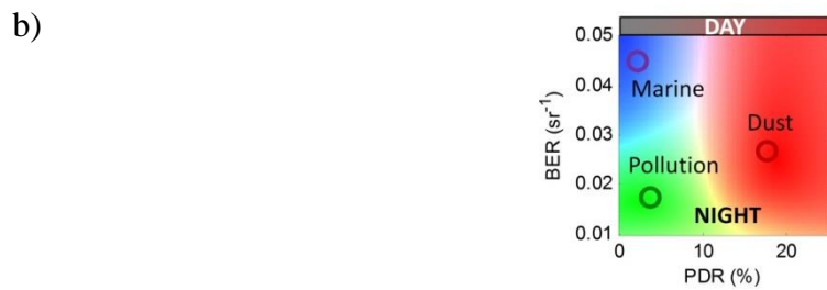
653 Figure 7: a) Results of aerosol speciation as given by lidar-derived extinction, PDR and BER, 654 with backscatter coefficient coded as saturation (no saturation, white = 0, full saturation = 5 655 10^{-6} \text{ m}^{-1} \cdot \text{sr}^{-1} ); b) Key for the colours of the above. Nighttime: dust-, pollution- and marine-like 656 aerosols coded as red, green and blue respectively. Daytime: PDR coded as the saturation of 657 red (top of the colour key). Intermediate colours and grey thus designate undetermined layers 658 where aerosol mixing may occur.
