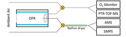
**Figure 1.** Simplified schematic of the experimental setup. Ambient air was alternately sampled either directly or through the oxidation flow reactor (OFR). In the OFR, the concentration of OH was increased to simulate atmospheric aging from hours up to several weeks.
