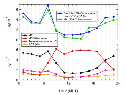
**Figure 11.** Top: diurnal maximum measured OA enhancement (all data from 0.4–1.5 eq. days aging, LVOC fate corrected) in the OFR from OH oxidation using the OFR185 method, and predicted OA formation from measured VOCs ( $\times$ 5.9). Bottom: ambient MT, SQT ( $\times$ 5), toluene + p-cymene ( $\times$ 5), and MBO + isoprene concentrations vs. time of day.
