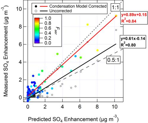
Figure 6. Measured vs. predicted SO<sub>4</sub> formation after OH oxidation in an OFR. The data points
