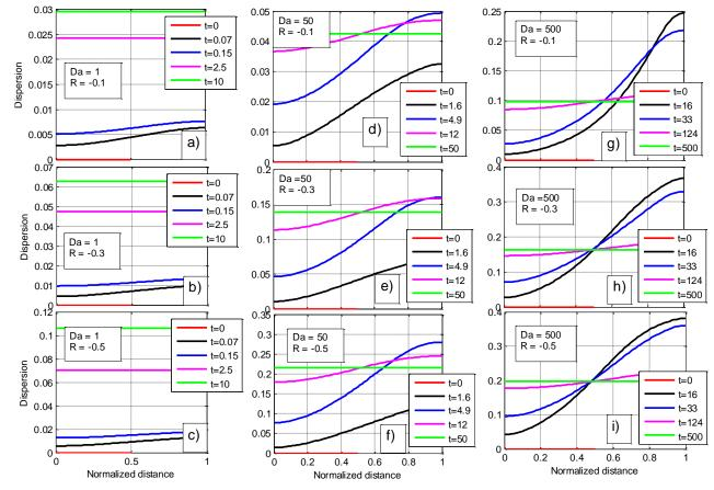
**Fig. 13.** Spatial dependencies of the relative DSD dispersion at different time instances and 1302 at different values of *Da* and different R > -1
