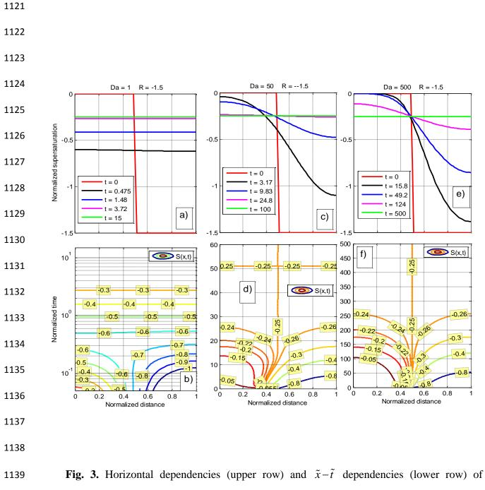
normalized supersaturation at Da = 1, Da = 50 and Da = 500 and at R = -1.5. Panel b is plotted in semi-log scale.
