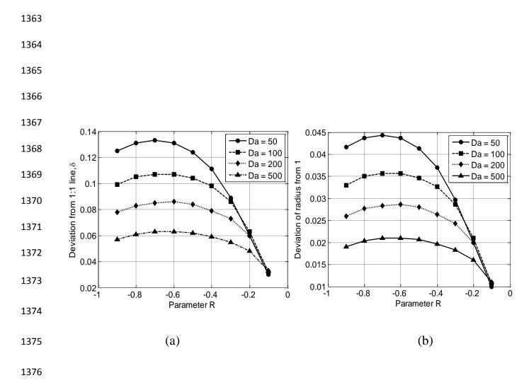
**Fig 17.** (a) Dependencies of the r.m.s. distance of the  $\tilde{N} - \tilde{q}$  relationship curve from straight line 1:1 suggested by classical concept of extremely inhomogeneous mixing. The dependencies are plotted for different values of *Da* and *R*. (b) The same as to the left panel but for r.m.s. deviations of the mean volume radius curve from that initial constant value assumed in the classical concept.
