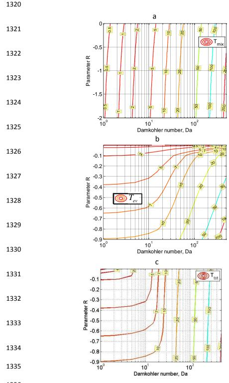
**Fig. 15.** Contours of normalized mixing duration times on Da - R plane. (a) mixing time  $T_{mix}$ , (b) evaporation time  $T_{ev}$ , and (c) the total duration mixing time  $T_{tot}$ .
