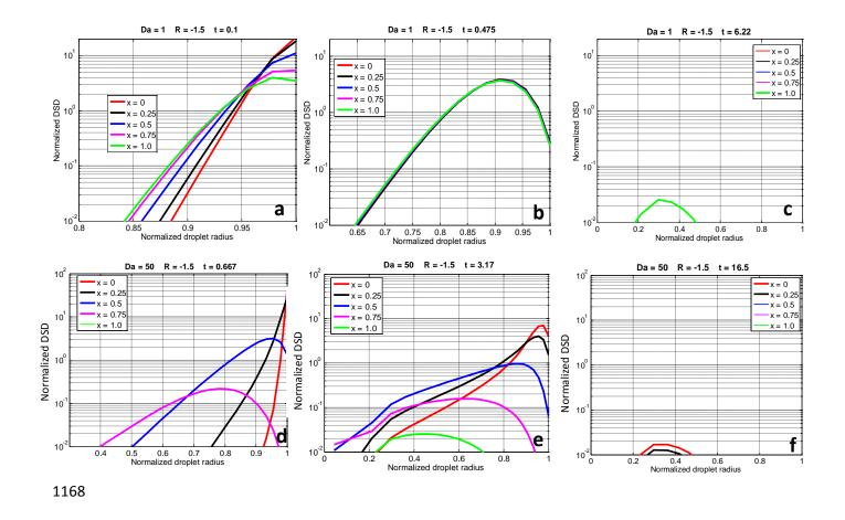
**Fig. 6** Time evolution of DSD during droplet evaporation at Da = 1 (upper row) and 1171 Da = 50 (bottom row). In each panel, the normalized DSD are shown at different values of 1172 horizontal coordinate  $\tilde{x}$ . Different panels show DSD at different time instances.
