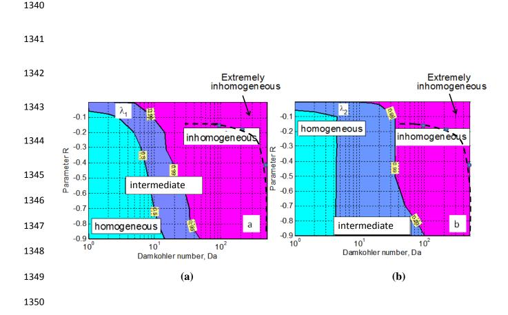
1351 Fig. 16. (a) The boundaries between mixing types on the Da - R plane designed according 1352 to criteria  $\lambda_1 = \frac{T_{mix}}{T_{tot}}$ ; (b) The boundaries between mixing types on the Da - R plane designed
