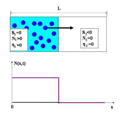
**Fig.1.** The schematic illustration of the 1D mixing problem considered in the study. The initial state at t = 0 is illustrated. The left volume of length L/2 is a saturated cloudy volume; the right volume is a non-saturated air volume from the cloud environment.
