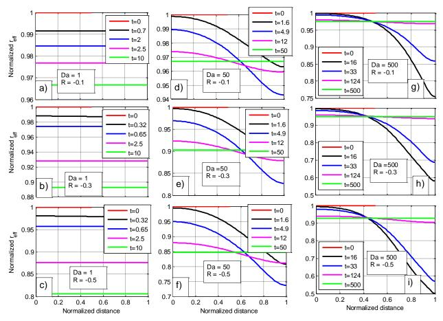
1310 Fig. 14. Spatial dependencies of the effective radius at different time instances and at 1311 different values of *Da* and different R > -1
