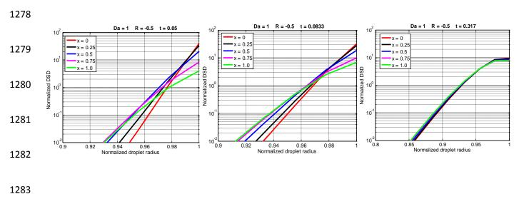
1287 Fig. 12. DSD at different  $\tilde{x}$  at the beginning of the mixing process for Da = 1 and 1288 R = -0.5.
