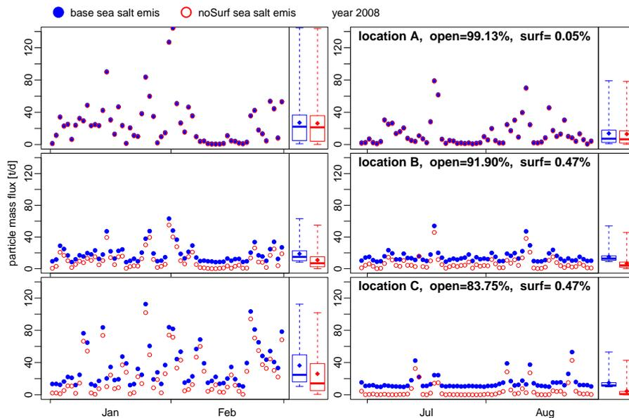
**Figure 4.** Daily averaged sea salt emission flux in  $t/d$  in three exemplary coastal grid cells (one per row) in winter 2008 (left) and summer 2008 (right). The fraction of open ocean and surf zone is listed in the plots on the right. The remaining share is land. Location A is located on the Dutch coast, location B is on the German coast and location C is on the Norwegian Atlantic coast.
