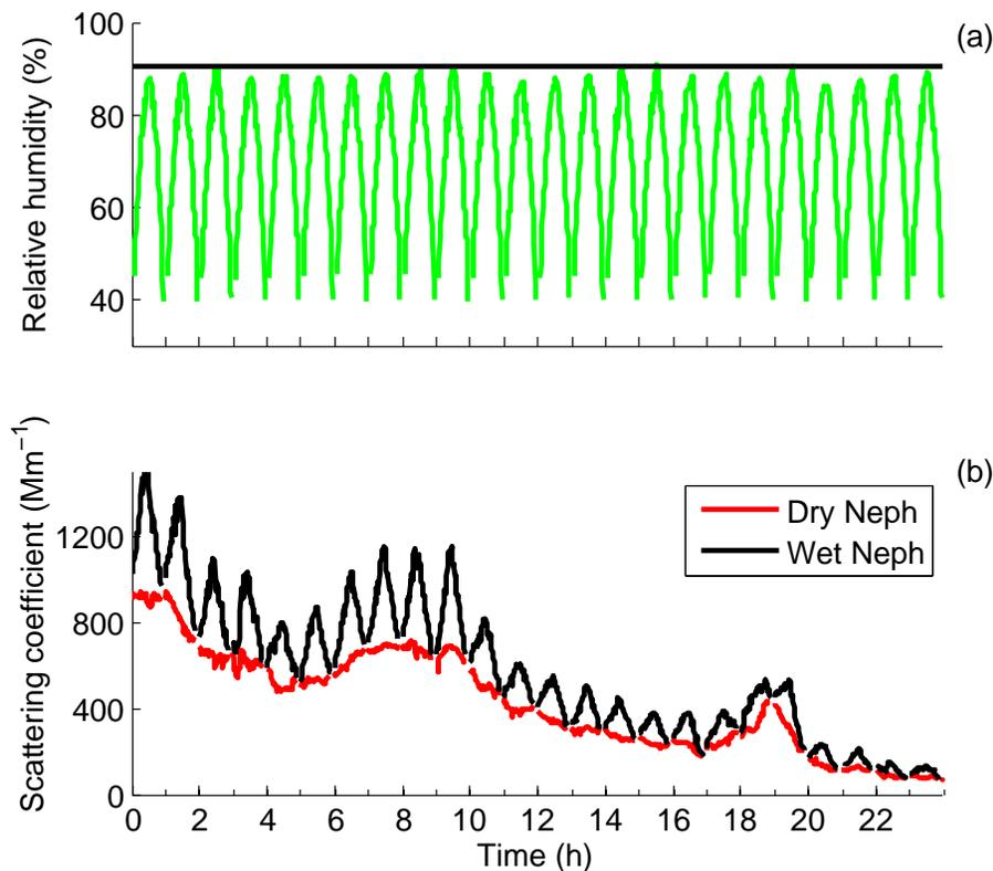
**Figure 3.** Example of recorded data on 17 March 2013 **(a)** Relative humidity of WetNeph, the black line represents  $RH = 91\%$ ; **(b)** Aerosol scattering coefficients measured by DryNeph (red line) and WetNeph (black line).
