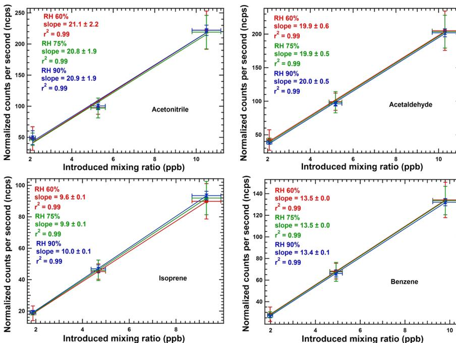
**Figure 3.** Compound specific normalized sensitivities at different relative humidities (RH 60, 75 and 90 %) for acetonitrile, acetaldehyde, isoprene and benzene during the calibration experiment performed on 10 January 2013. Horizontal bars reflect the error due to the MFC flows and the accuracy of the VOC gas standard whereas vertical bars reflect the precision error ( $2\sigma$ ) of the measurements.
