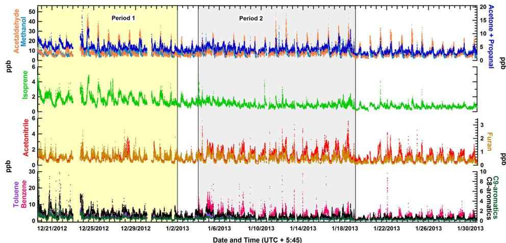
**Figure 4.** Time series of one minute time resolution data for the mixing ratios of methanol, acetaldehyde, and the sum of acetone and propanal (top panel); isoprene (second panel from top); acetonitrile and furan (second panel from bottom); benzene, toluene, the sum of C8-aromatics (xylene isomers and ethyl benzene) and the sum of C9-aromatics (isomers of trimethyl benzenes and propyl benzenes) (bottom panel) during SusKat-ABC campaign.
