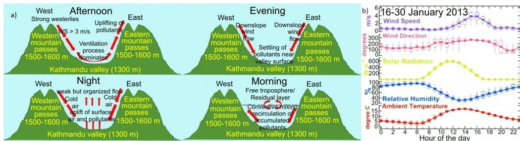
**Figure 2.** (a) Schematic of wind flow during different times of the day in the Kathmandu Valley. (b) Box and whisker plots of the measured meteorological parameters (wind speed, wind direction, solar radiation, relative humidity and ambient temperature) at the Bode site (16–30 January 2013).
