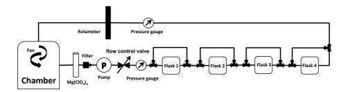
Figure 2. Scheme of the sampling setup using the closed-cycle air sampler. The volume of the soil chamber was 22.8 L and the volume of each flask was 1 L.
