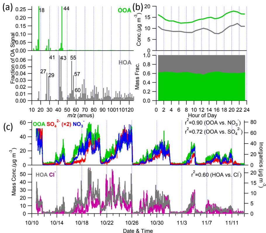
**Figure 4.** (a) Mass spectra of HOA and OOA, (b) diurnal variations of the mass concentration and mass fraction of HOA and OOA, (c) time series of HOA, OOA, and inorganic species ( $\text{SO}_4^{2-}$ ,  $\text{NO}_3^-$ ,  $\text{Cl}^-$ ). The correlations of HOA and OOA with inorganic species are also shown in the figure.
