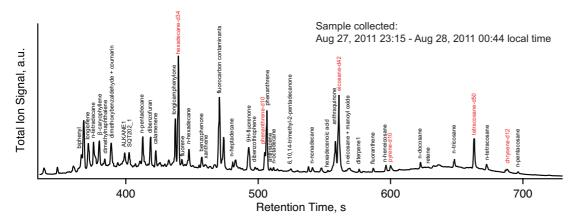
**Figure 2.** Total ion chromatogram of a typical sample. Deuterated internal standards (labeled in red) were injected prior to thermal desorption. The labeled compounds represent a subset of the compounds identified. More compounds were identified using the selected ion traces. A partial list of compounds tentatively identified is shown in Table 1, and the full list is shown in Table S1 in the Supplement.
