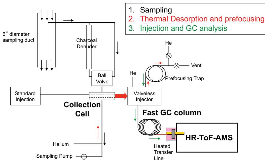
**Figure 1.** A schematic of the SV-TAG sample introduction system into the HR-ToF-AMS. The arrows in black, red, and green denote the flow paths during sample collection, thermal desorption and prefocusing, and injection into GC/MS analysis, respectively.
