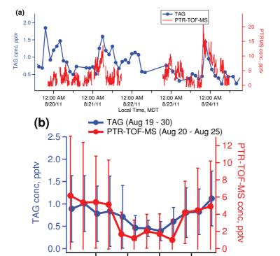
**Figure 4. (a)** Time series of SQT204 concentration measured by PTR-TOF-MS and by TAG during measurement overlap. **(b)** Diurnal profile of SQT204 concentration during the entire measurement period of TAG (19–25 August) and PTR-TOF-MS (20 July–25 August).
