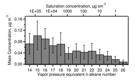
**Figure 5.** Average volatility distribution of total hydrocarbons observed by SV-TAG. The whiskers represent the standard deviation of the measurements.
