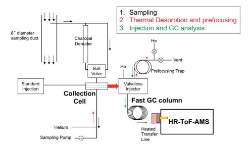
Figure 1. A schematic of the SV-TAG sample introduction system into the HR-ToF-AMS. The arrows in black, red, and green denote the flow paths during sample collection, thermal desorption and prefocusing, and injection into GC/MS analysis, respectively.
