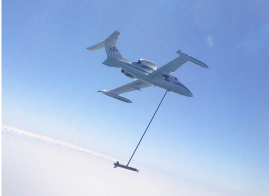
Figure 1. Photo from the Learjet 35A with towed AIRTOSS. The picture was taken during a test flight from a second aircraft.
