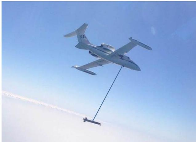
**Figure 1.** Photo from the Learjet 35A with towed AIRcraft TOWed Sensor Shuttle. The picture was taken during a test flight from a second aircraft.
