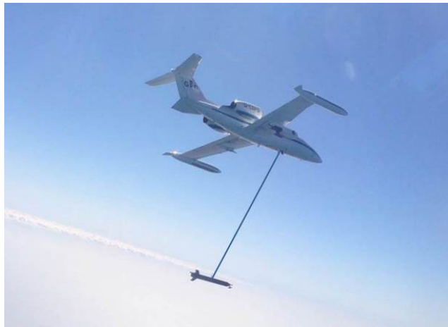
Figure 1. Photo from the Learjet 35A with towed AIRcraft TOWed Sensor Shuttle. The picture was taken during a test flight from a second aircraft. The cable was artificially thickened to make it visible in the photo.
