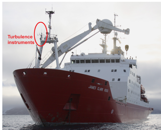
Figure 1. Locations of the flux instrumentation on the RRS James Clark Ross . Note that the forecandle crane is generally stowed close to the deck while the ship is underway or on station.
