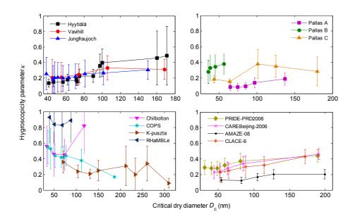
**Figure 6.** Mean hygroscopicity parameter  $\kappa$  as a function of critical dry diameter  $D_c$  for selected locations. Figure split in four panels for more detail. Shown with one standard deviation.
