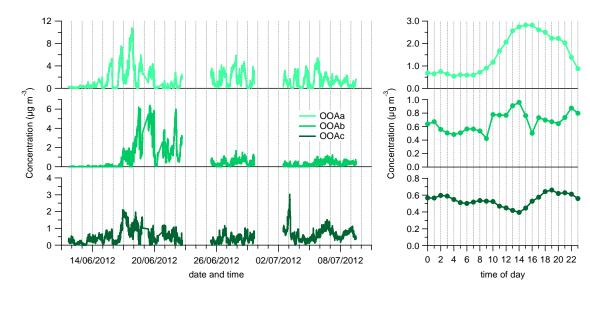
3 Figure 9. Time series and diurnal trend of the three factors extracted by PMF.
