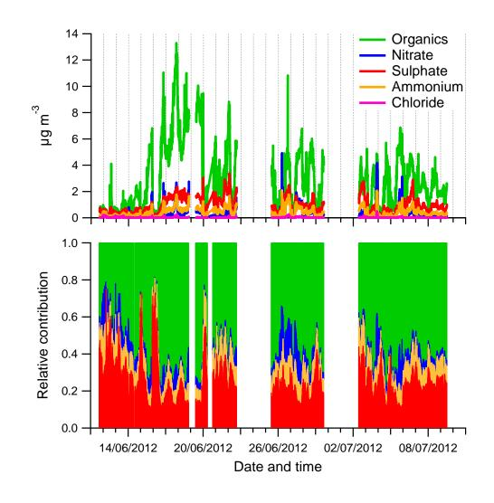
3 Figure 1. Time series and relative contribution of the main NR-PM<sub>1</sub> components. Time is
