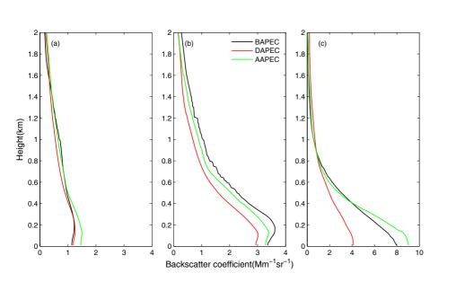
**Figure 7.** Backscattering profiles under different pollution conditions during the periods of BAPEC, DAPEC and APPEC (a)  $PM < 50 \,\mu g \,m^{-3}$ , (b)  $50 \,\mu g \,m^{-3} < PM < 100 \,\mu g \,m^{-3}$ , (c)  $PM > 100 \,\mu g \,m^{-3}$ .
