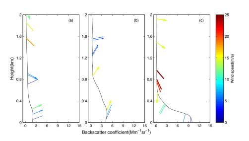
**Figure 13.** Attenuated backscattering coefficient profile and wind profile during the heavy pollution process for 17–21 November at (a) 20:00 LT on 17 November, (b) 20:00 LT on 18 November, (c) 20:00 LT on 21 November.
