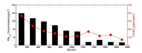
Figure 2. PM<sub>2.5</sub> concentrations and CO/SO<sub>2</sub> ratios of the mixing layer at different heights.
