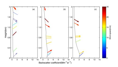
**Figure 11.** Attenuated backscattering coefficient profile and wind profile during the heavy pollution process for 6–11 November at (a) 20:00 LT on 7 November, (b) 20:00 LT on 8 November, and (c) 20:00 LT on 10 November.
