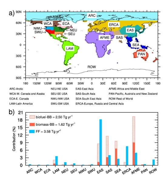
**Fig. 1.** (a) Tagged source regions and (b) the contributions (%) to the global mean BC emissions (7.69 Tg yr<sup>-1</sup>) for January, February and March from the individual source regions (marked on the horizontal axis) and sectors (FF in blue, biomass-BB in solid red, and biofuel-BB in dotted red).
