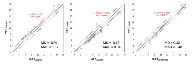
This figure reveals that the discrepancies between the three prediction techniques for the  $\alpha$ -pinene oxidation products, when expressed as MDs and MADs, are of a similar size (in the case of the comparisons involving the SPARC predictions) or slightly larger (in the case of the COSMOtherm vs. ppLFER comparison) than those discrepancies for the n-alkane oxidation products. In particular, the mean difference is smaller than one log unit in all three cases.
